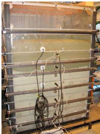
They instrumented a tank with RH and Echo sensors, tensiometers and psychrometers to compare results, and found “*the response of the TP sensor has been found to be in agreement with that of suction measurement, while the response of the ECH2O-TE showed some anomalies*”.
