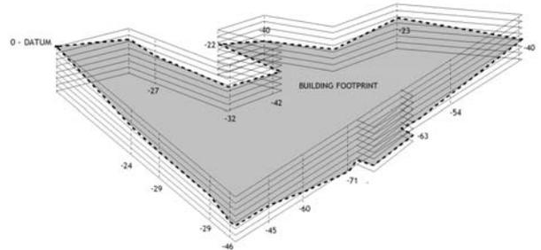
Above is a 3D distortion profile relating to readings taken in October, 2009. Below is the plot of the speed of recovery over time using linear trendlines.
