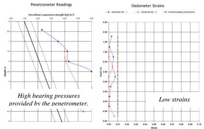
High bearing pressures provided by the penetrometer.
